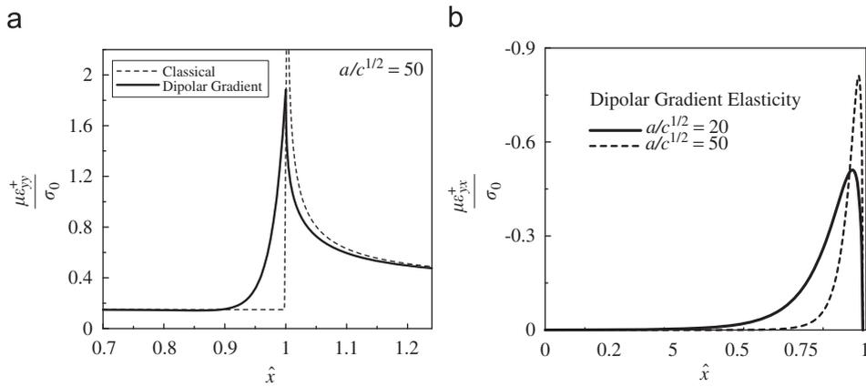
Fig. 6. Distribution of (a) the normal strain  $\epsilon_{yy}$  and (b) the shear strain  $\epsilon_{yx}$  of the upper crack face in classical and dipolar elasticity. Poisson's ratio is  $\nu = 0.3$ .
