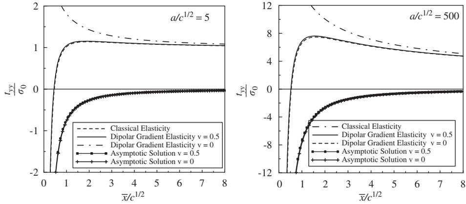
Fig. 4. Distribution of the total normal stress ahead of the crack tip for two different values of the ratio  $a/c^{1/2}$  and for Poisson's ratios  $\nu = 0$  and  $0.5$ .
