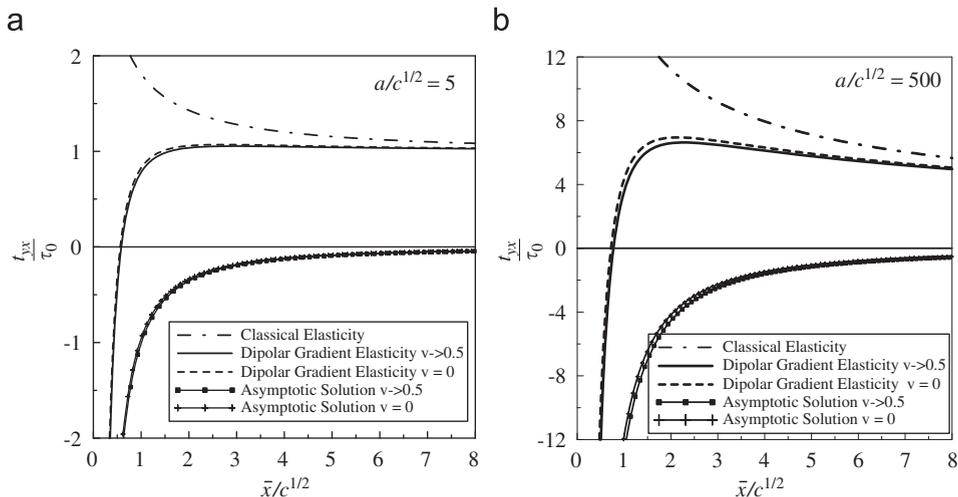
Fig. 9. Distribution of the total shear stress ahead of the crack tip for two different values of the ratio  $a/c^{1/2}$  and for Poisson’s ratios  $\nu = 0$  and  $0.5$ .
