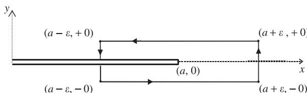
Fig. 10. Rectangular-shaped contour surrounding the RHS crack-tip.
