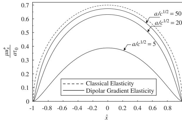
Fig. 8. Profiles of the normalized crack sliding displacement ( $\mu_x^+/\sigma_0$ ) of the upper face along the entire crack line. Poisson’s ratio is  $\nu = 0.3$ .
