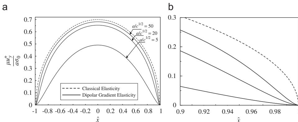
Fig. 3. Profiles of the normalized crack opening displacement ( $\mu u_y^+ / a\sigma_0$ ) of the upper face (a) along the entire crack line, and (b) near to the RHS crack tip. Poisson's ratio is  $\nu = 0.3$ .
