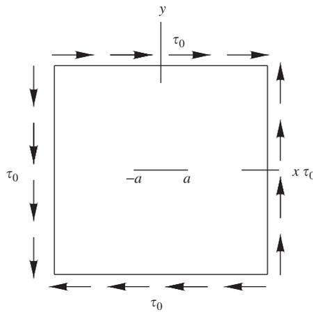
Fig. 7. Cracked body under remote shear in plane strain.
