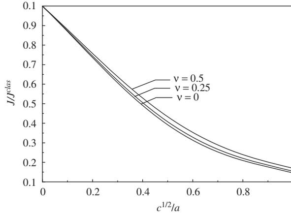
Fig. 11. Variation of the  $J$ -integral for the mode I case in dipolar gradient elasticity with  $c^{1/2}/a$ .
