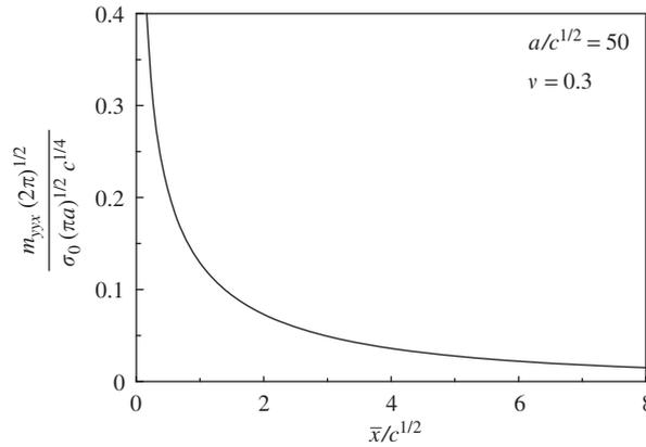
Fig. 5. Distribution of the dipolar stress ahead of the crack tip.
